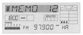
If the station is not yet stored, the display will show \* NEW. Because of the large capacity of the memory, this indication appears only after approx. 1 second.
