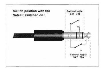
The switching circuit for controlling the cassette recorder operates "potential-free" (relay control).
